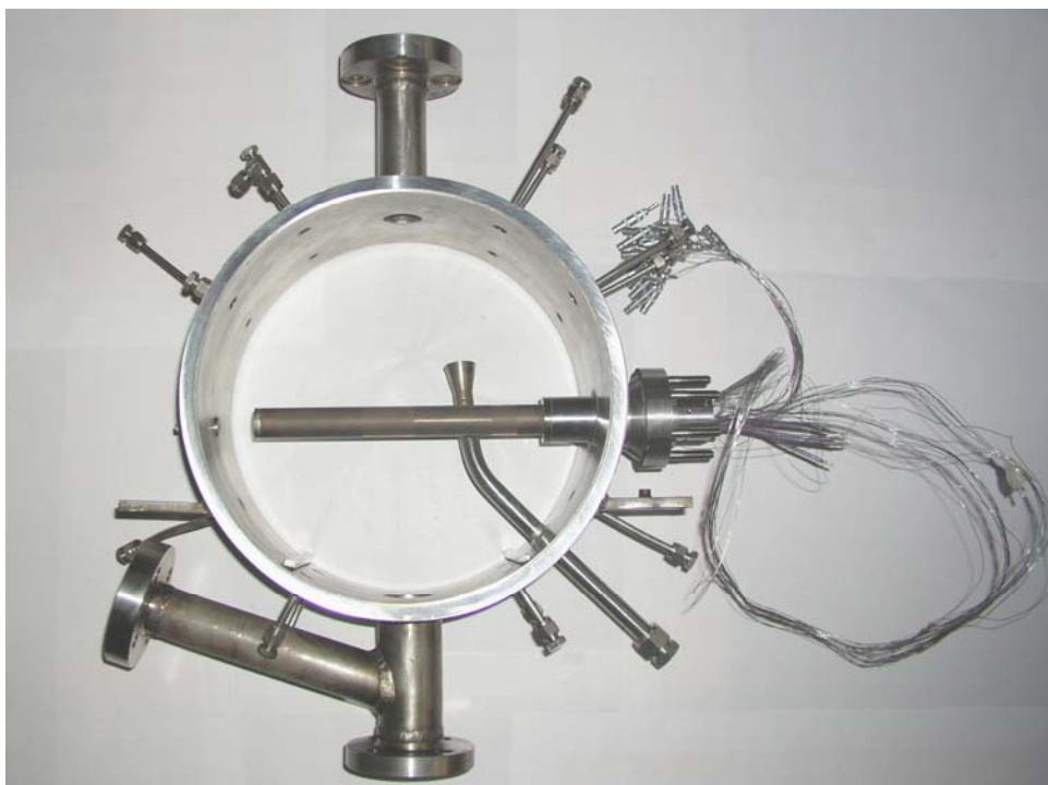
Figure 3: Photo showing the open evaporator with a mounted test tube. The thermocouples installed in the test tube allow for wall temperature measurements with high peripheral resolution. The premixed feed enters the pool at the bottom. Vapor leaves the evaporator at the top. Liquid for the circulation loop is withdrawn from a level above the test tube through the tube installed on the right side of the evaporator.
